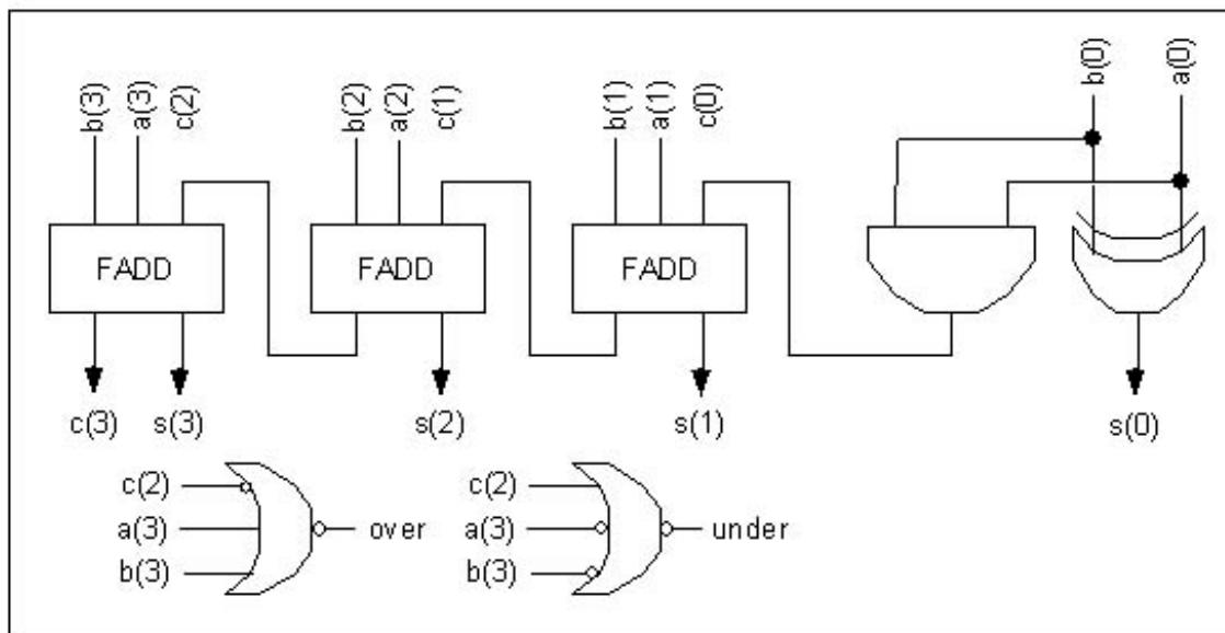
Underflow occurs when adding two negative numbers, the result is positive number. This happens when  $a(3)=b(3)=1$ , and no previous carry,  $c(2)=0$ . Overflow occurs when adding two positive number, the results is a negative number. This happens when  $a(3)=b(3)=0$ , and with previous carry ,  $c(2)=1$ .
