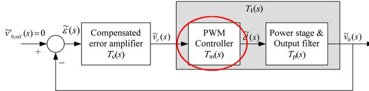
$$T_m(s) = \frac{\tilde{d}(s)}{\tilde{v}_c(s)} = \frac{1}{\hat{V}_r} \Rightarrow T_1(s) = \frac{\tilde{v}_o(s)}{\tilde{v}_c(s)} = \frac{\tilde{v}_o(s)}{\tilde{d}(s)} \frac{\tilde{d}(s)}{\tilde{v}_c(s)} = T_p(s) T_m(s)$$
