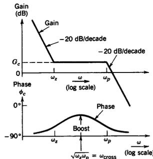
$$T_c(s) = \frac{1}{R_1 C_2 s} \frac{s + \omega_z}{s + \omega_p}$$
