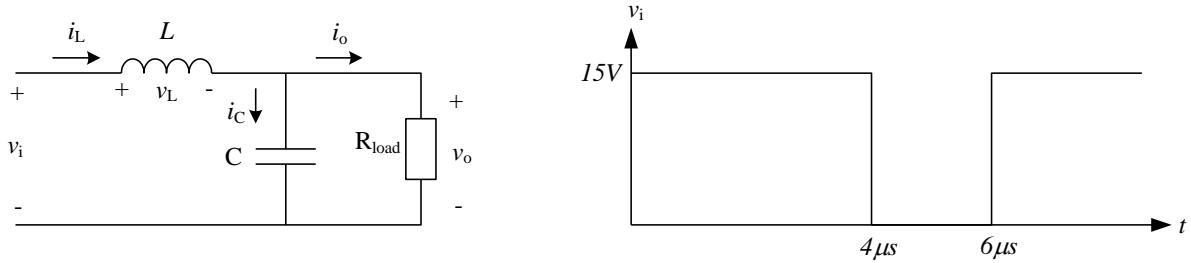
The applied voltage ( $v_i$ ) is repetitive and the system is in steady state. Assume that the capacitance is very large, the inductor has a value of  $L = 5\mu H$  and that the load consumes 250W ( $P_{load}$ )
