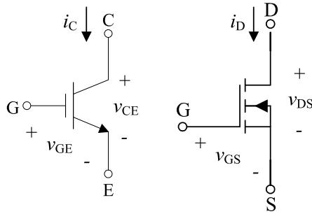
(a) Sketch the voltages ( $v_{CE}$  and  $v_{DS}$ ) over the two switching devices as function of the current through the devices ( $i_C$  and  $i_D$ ).
