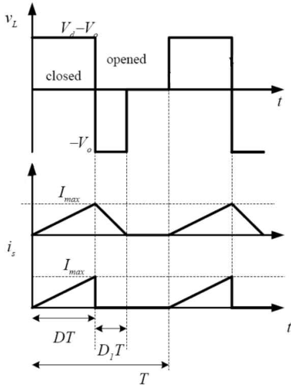
The ratio between input and output voltage can be calculated via the average inductor voltage:
