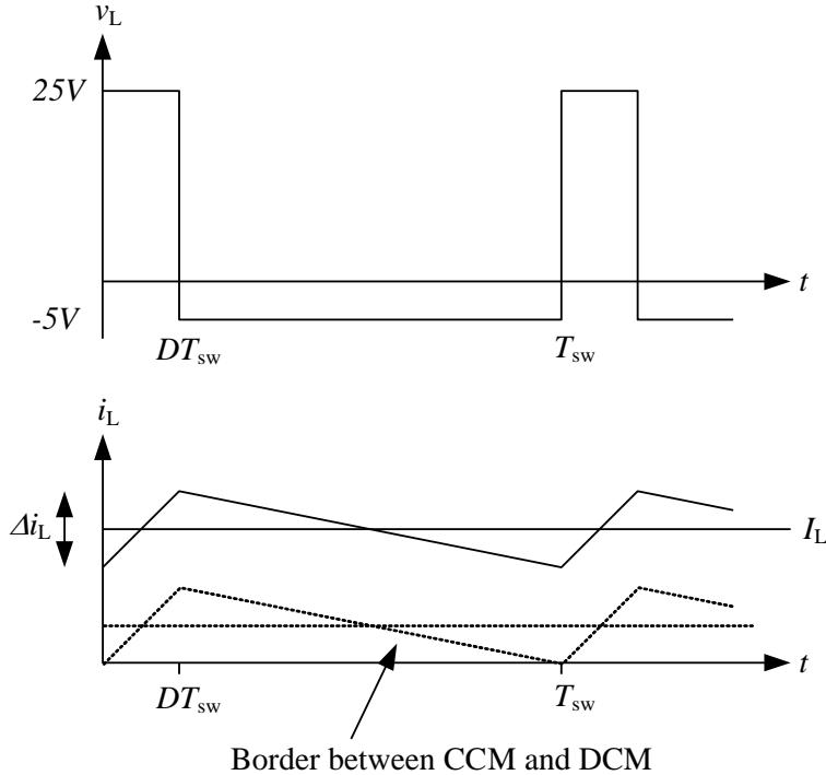
Since  $v_L$  and  $L$  are constant the derivative of the inductor current must be constant. This gives a linear increase and decrease of the inductor current.
