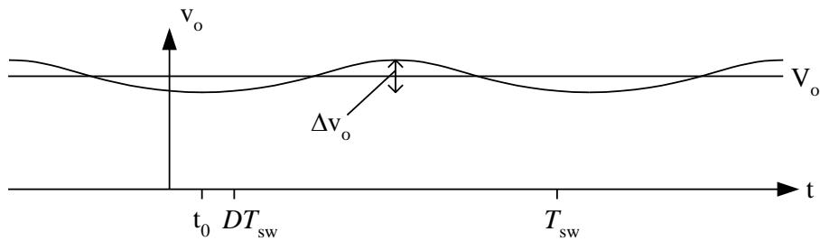
We don't have to solve this because we are only interested of finding the peak-to-peak ripple in the output voltage. From the figure we see that from the time  $t_0$  the capacitor current is positive to time  $t = t_0 + T_{sw}/2$ . This gives that the capacitor voltage will increase from time  $t_0$  to time  $t = t_0 + T_{sw}/2$ . The peak-to-peak ripple in the output voltage can then be calculated by
