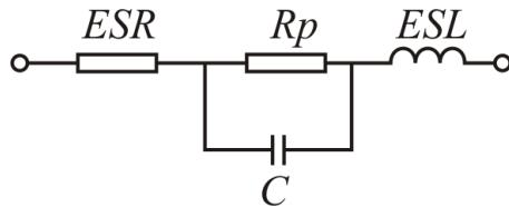
ESR is the equivalent series resistor, ESL is the equivalent series inductance and  $R_p$  is the parallel resistor that causes leakage current.
