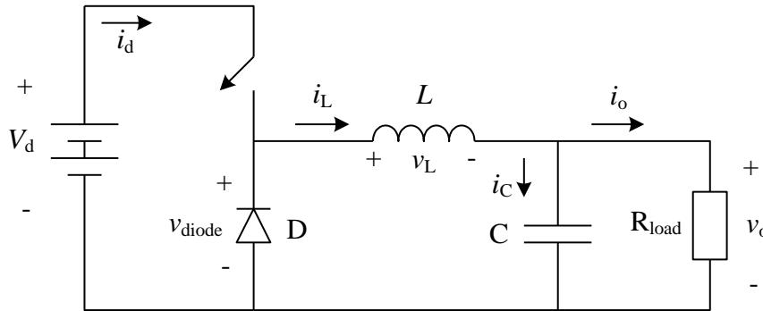
In a step-down converter consider all components to be ideal. Let the output voltage be held constant at 5V by controlling the switch duty ratio D. The input voltage ( $V_d$ ) is 30V, the switching frequency ( $f_{sw}$ ) is 50 kHz, the inductance is 100  $\mu$ H, the capacitance is 470  $\mu$ F and the output power is 40W. Ignore the forward voltage drop on the diode.
