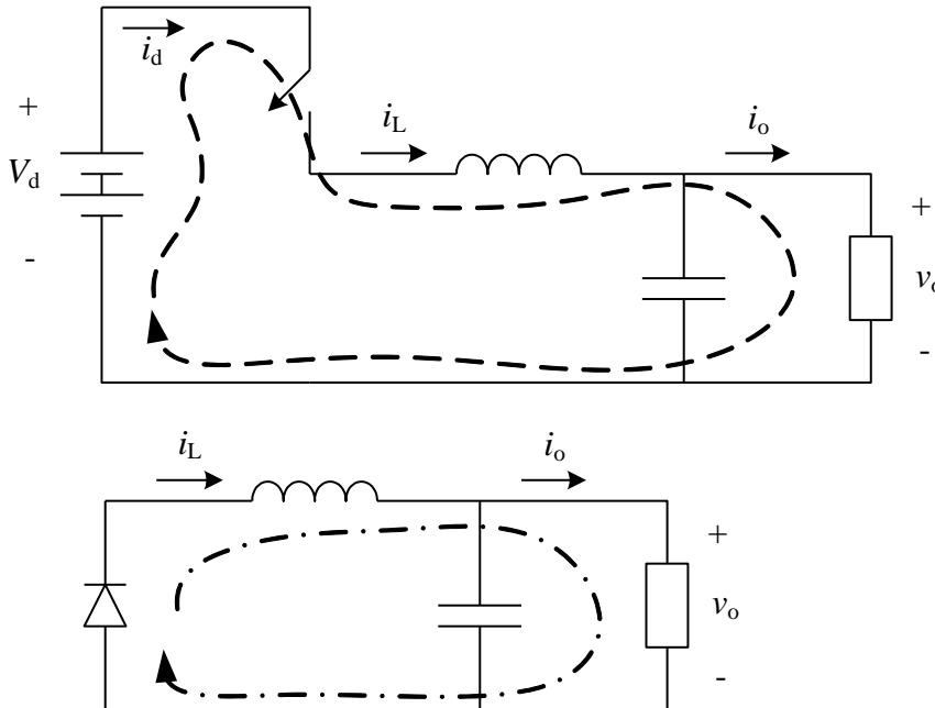
Since we have assumed a large output capacitor, the output voltage is assumed to be a constant DC-voltage. When the switch is turned on, the inductor voltage becomes:  $v_L = V_d - V_o$ . When the switch is off, the inductor voltage becomes:  $v_L = -V_o$ .
