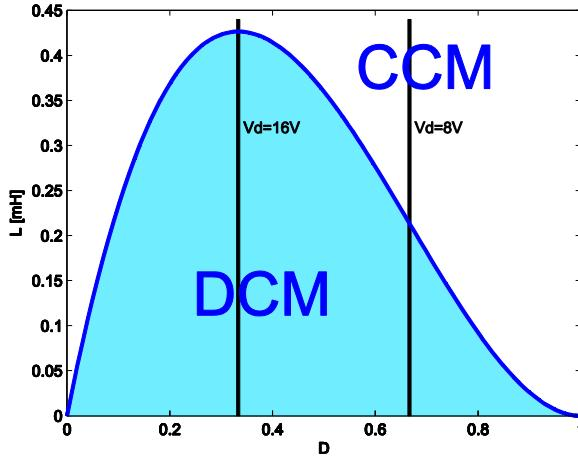
The lowest output power gives the highest inductance, this gives that  $P_o = 5W$ . For the given operating conditions ( $V_o = 24V$  and  $V_d$  varies between 8V and 16V), the following expression for the duty-ratio applies:
