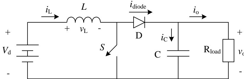
We assume that the converter is in steady state and that the output capacitor is so large that the output voltage can be treated as a DC voltage.
