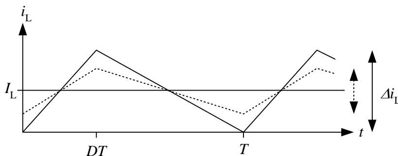
From the figure it can be seen that the converter is operating in CCM if  $I_L \geq \Delta i_L/2$ . If the average value of the inductor current is equal to half the peak-to-peak ripple in the inductor current, the converter will be operating at the border between DCM and CCM, see the solid line in the figure. If the ripple is reduced there will be a margin to the border, see the dashed line.
