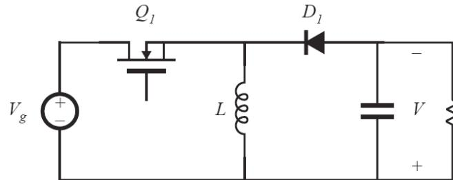
The derivation of a flyback converter comes from the buck-boost converter. The figure above depicts the basic buck-boost converter, with the switch realized using a MOSFET and diode. The converter is changed so that the inductor winding is constructed using two wires, with a 1:1 turns ratio. The basic function of the inductor is unchanged, and the parallel windings are equivalent to a single winding constructed of larger wire.
