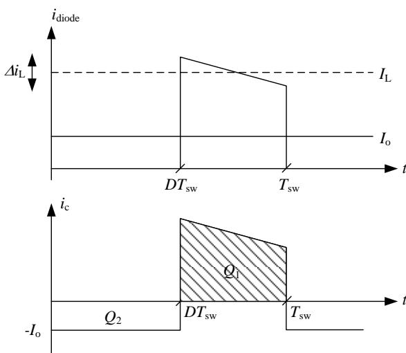
When the capacitor current is positive, charge is added to the
