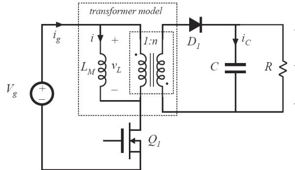
The magnetizing inductance  $L_M$  functions in the same manner as inductor  $L$  of the original buck-boost converter. When transistor  $Q_1$  conducts, energy from the dc source  $V_g$  is stored in  $L_M$ . When diode  $D_1$  conducts, this stored energy is transferred to the load, with the inductor voltage and current scaled according to the  $1:n$  turns ratio.
