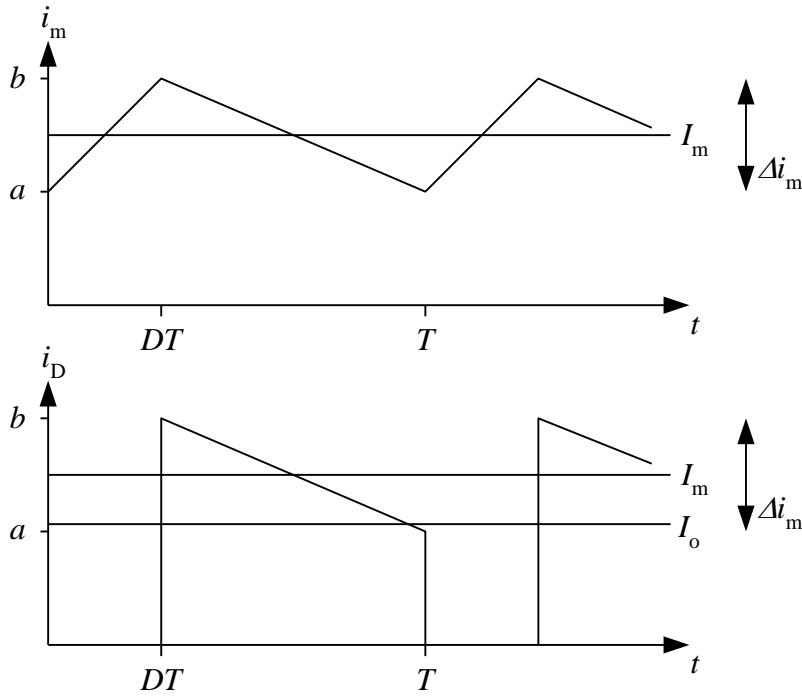
From the figure we see that the average magnetizing current can be calculated as:
