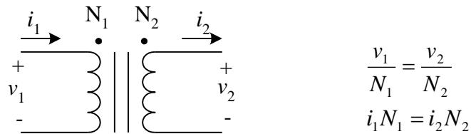
If we apply a positive voltage at the dot then we get a positive voltage at the dot on the other side. If we have a current going in at the dot we must then have a current going out from the dot on the other side. If not, we would put in power from both sides, which mean that no power is transferred. This is not possible since we are studying an ideal transformer.
