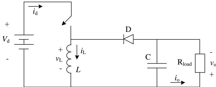
$$V_d = 12V \quad V_o = 15V \quad f_{sw} = 20kHz \quad C = 470\mu F$$
