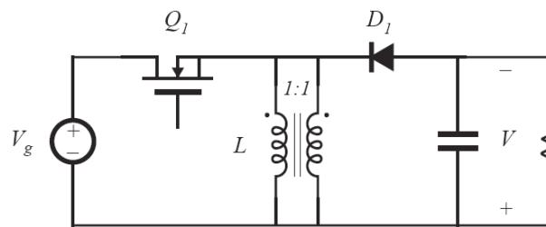
In next step, the connections between the two windings are broken. One winding is used while the transistor  $Q_1$  conducts, while the other winding is used when diode  $D_1$  conducts.
