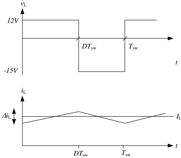
$$\Delta i_L = \frac{V_d D}{f_{sw} L} = \frac{12V \cdot 0.556}{20kHz \cdot 350\mu H} = 0.95A$$
