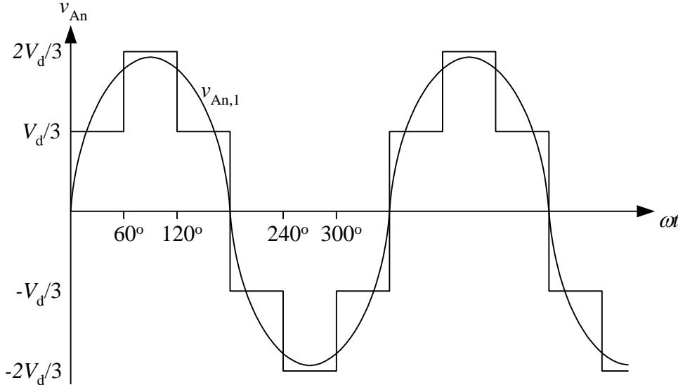
We know that the back-emf voltage ( $e_A = e_B = e_C$ ) is a sinusoidal voltage with the same frequency as the fundamental. We also know that:
