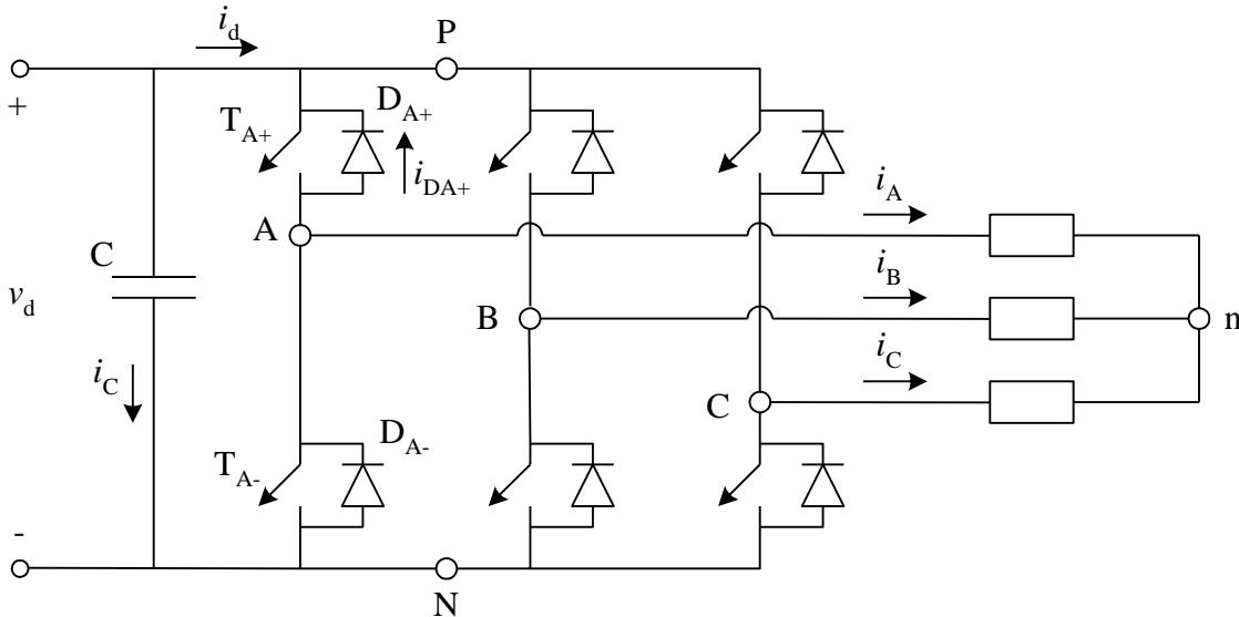
Draw the steady state waveforms for  $v_{An}$ ,  $i_A$ ,  $i_{DA+}$  and  $i_d$ , where  $i_{DA+}$  is the current through diode  $D_{A+}$ .
