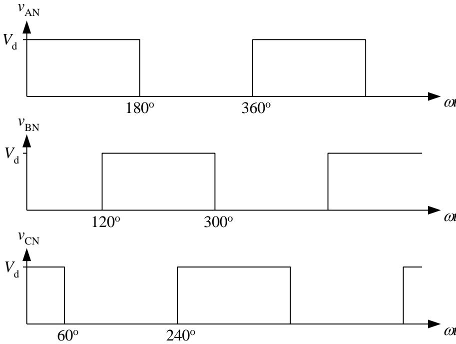
The load is assumed to be balanced ( $L_A = L_B = L_C$ ), which gives that the sum of the back-emf's must be equal to zero:
