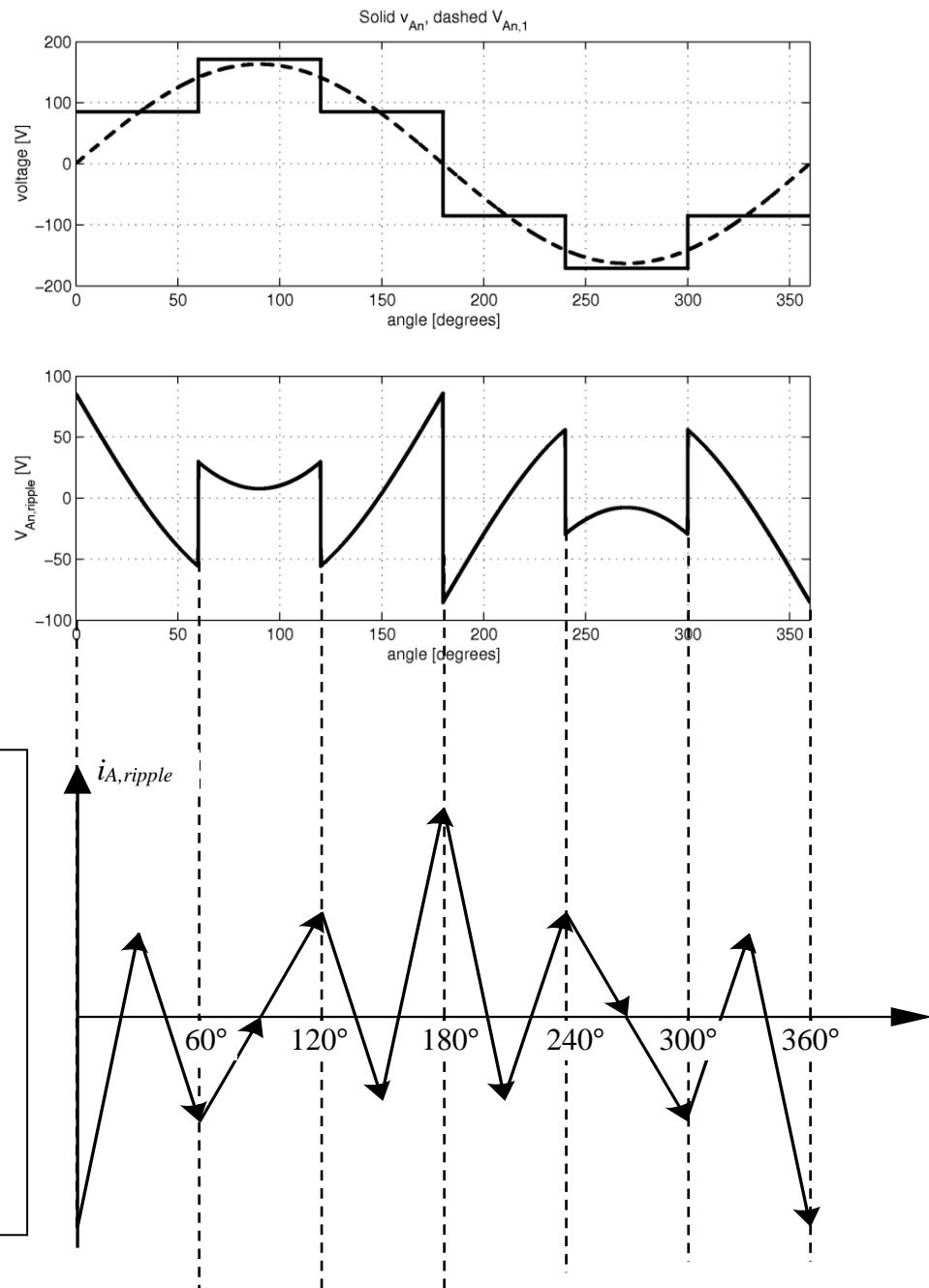
From the figures we see that we have symmetry lines at  $90^\circ$ ,  $180^\circ$  and  $270^\circ$ . We see that the ripple voltage is odd around  $180^\circ$  ( $v_{An,ripple}(180 - \theta) = -v_{An,ripple}(180 + \theta)$ ,  $\theta \geq 0$ ). This leads to a ripple current that is
