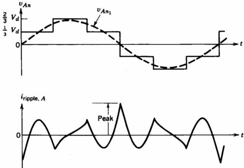
Now we know a starting point for solving the differential equation ( $i_{A,ripple}(90^\circ) = 0A$ ) and we also know that the maximum ripple current occurs at  $\theta = 180^\circ$ . We now calculate the peak ripple current:
