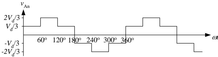
Note that the voltage in each phase has the same amplitude, but with the only difference that they are  $120^\circ$  phase shifted. Since we have a purely resistive load, the current has the same shape as the voltage.
