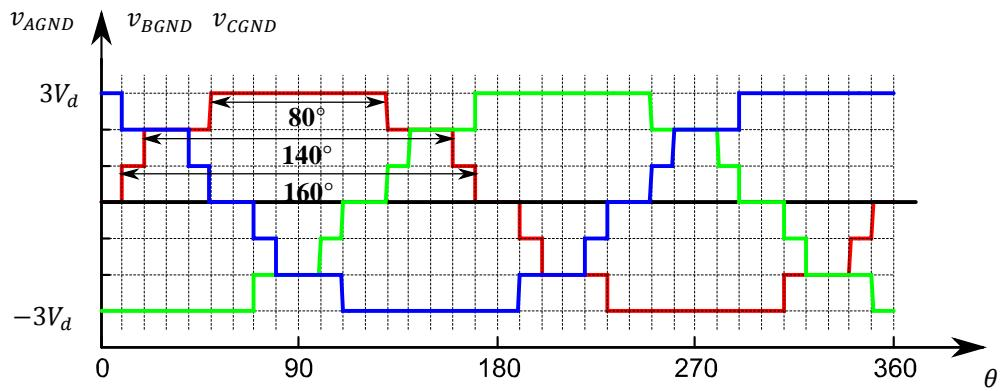
The line to line voltage,  $v_{AB}$ , can be drawn as the difference between the two phase potentials with respect to GND above as
