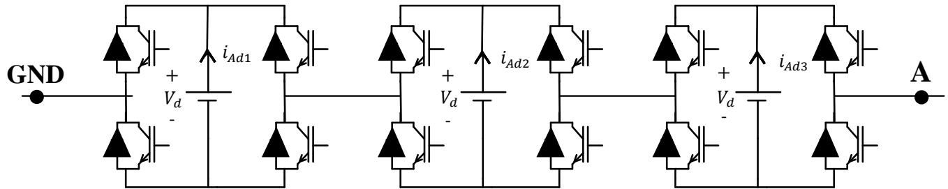
Due to the resistive load, the phase current will have the same shape as the phase voltage. The currents from the DC-sources will always be positive as active power is supplied to the load. If the same source is assumed to supply during the same interval during a full period (both half periods are the same), the three different source currents can be drawn as
