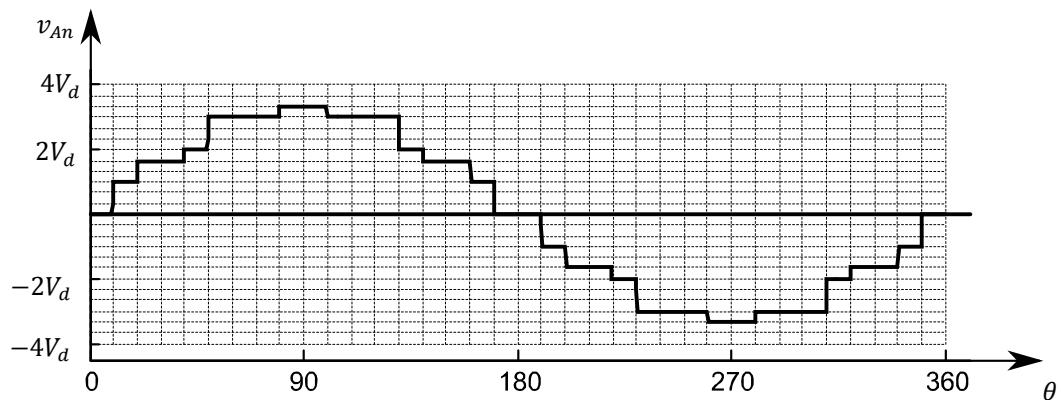
Please, observe the phase shift of  $30^\circ$  between the phase voltage and the line to line voltage (which was also shown in Demonstration 1).
