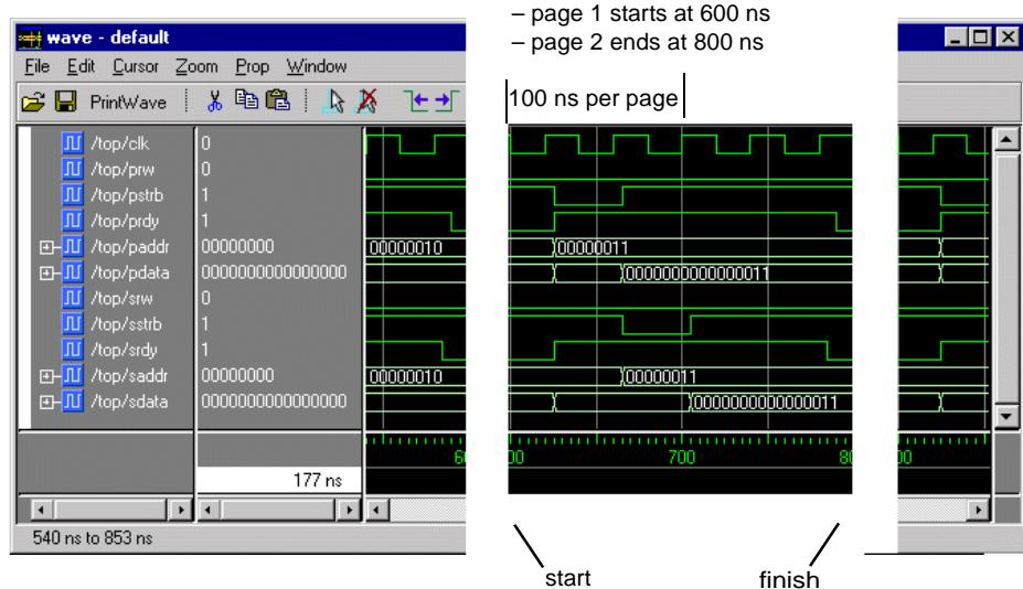
To make the job of creating a PostScript waveform output file easier, use the **File > Print Postscript** menu selection in the Wave window. See "[Printing and saving waveforms](#)" (UM-276) for more information.
