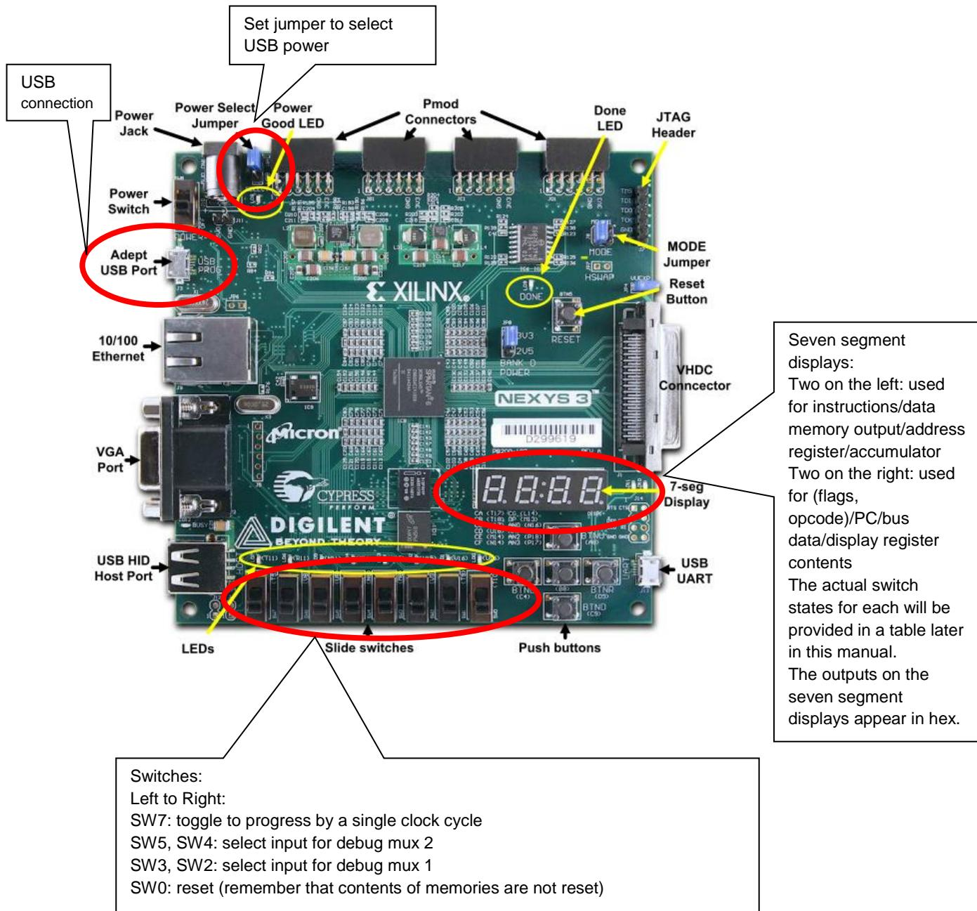
The VHDL modules provided to you for use in this lab contain code which allows you to display values on certain top level ports onto one of two pairs of seven segment displays available on the board. The choice is made using switches SW2 through SW5. The table below shows how the state of these switches affects outputs on the seven segment displays.
