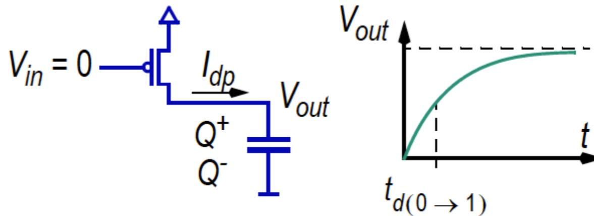
$$t_{d(0 \rightarrow 1)} = \frac{C_L}{k \cdot V_{DD}}$$
