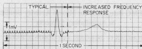
Fig. 8. Interference from a fluorescent light source on an ECG recording. Typical and increased frequency response shown.
