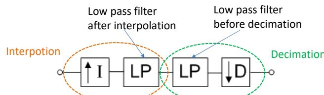
It is obvious that we can leave out one of the low pass filters and only keep the one with the lowest cut off frequency
