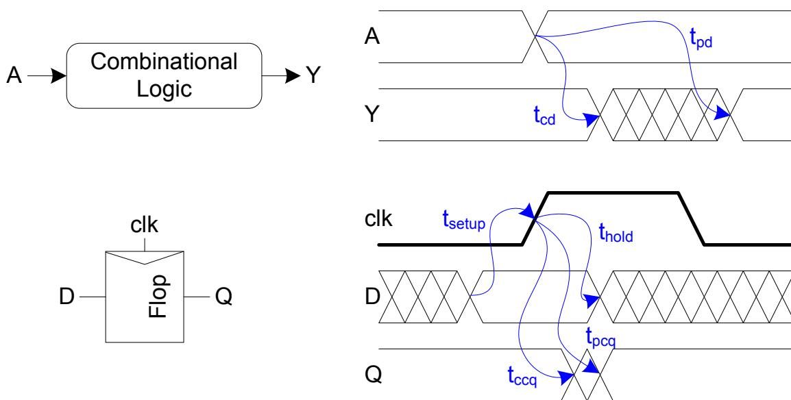
You are to use this type of flip-flops for sequencing in a system. Your task is to design the combinational logic, CL, which is to be placed between the flip-flops; therefore you need to determine the timing constraints for this logic.
