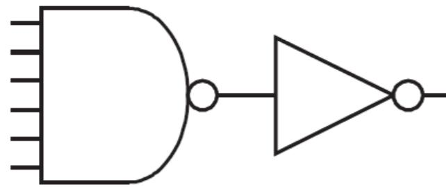
$$\begin{aligned} g_{\text{NAND4}} &= 2 & g_{\text{INV}} &= 1 \\ p_{\text{NAND4}} &= 8/3 & p_{\text{INV}} &= 1 \end{aligned}$$
