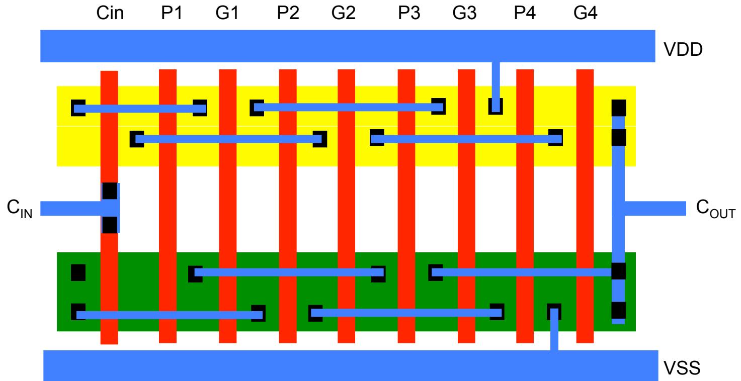
The layout is very compact and elegant, however, only post-layout circuit simulations with node capacitances extracted from the layout will reveal the exact performance of the cell.
