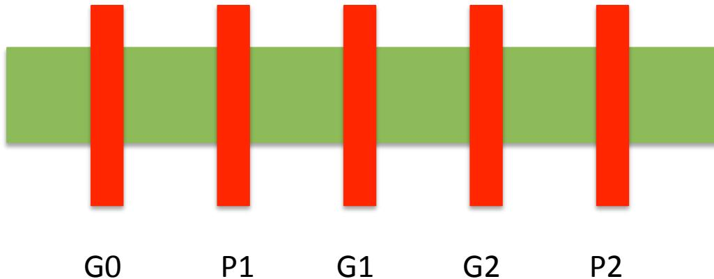
To map Euler path to a continuous line of diffusion start by labeling the transistors with their signal name starting at one end of Euler path.
