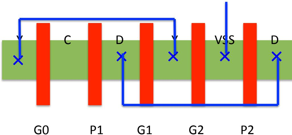
The make the connections for the source-drain areas that have the same circuit-node label.
