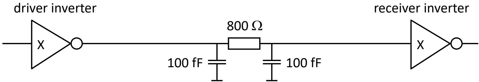
The given parameters yield a wire resistance of  $800 \Omega$  and a wire cap is  $200 \text{ fF}$ . Wire resistance is distributed along the wire which must be modeled by segments. In Spice circuit simulations a 3-segment  $\pi$ -model is accurate to within 3%. However, for simple analytical estimate: use single segment  $\pi$ -model.
