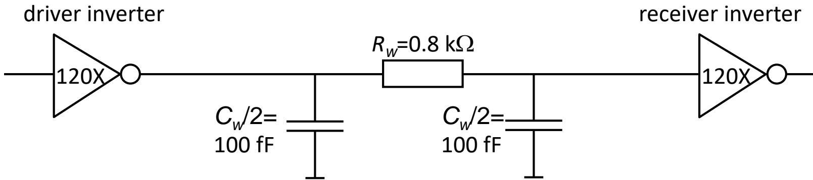
Having defined inverter size  $10X$  for inverters with  $R=2 \text{ k}\Omega$ ,  $120X$  is the inverter size with  $R_{eff}=170 \Omega$  minimizing the delay caused by the wire.
