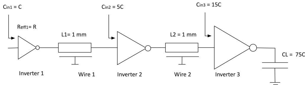
a) The capacitance of the entire wire is  $2000 * 0.05C = 100C$ . That is each 1-mm wire has a capacitance that is  $50C$ . The resistance of the entire wire is  $2000/0.2$  (number of squares) \*  $0.0001 R = R$ ; that is each 1-mm wire has a resistance that is  $R/2$ .
