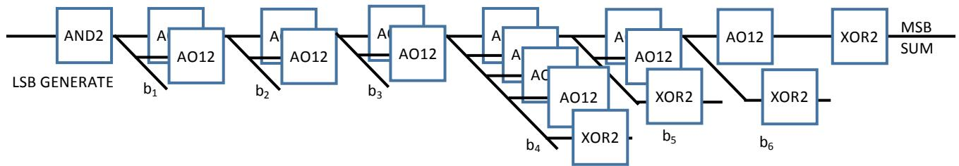
The total relative delay for this critical path is (neglecting the XOR gates for the sum calculations):
