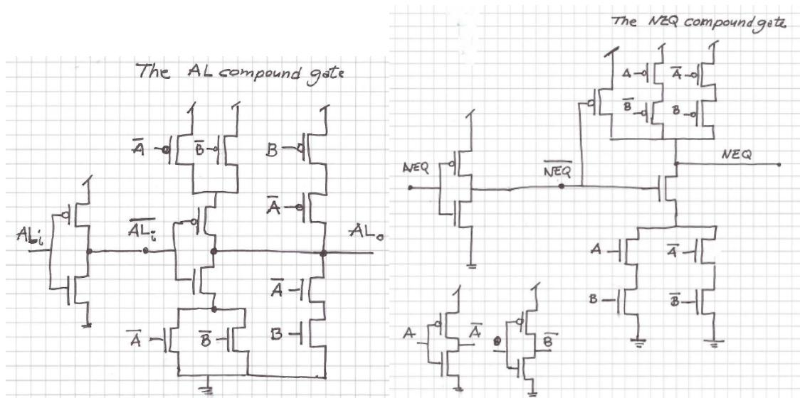
c) The setup can be seen below. The input value for the first ALi signal does not matter but the NEQi signal of the LSB cell must be set to 0. Only if all cells fulfill the propagate condition does the 0 appear at the NEQ output of the last cell.
