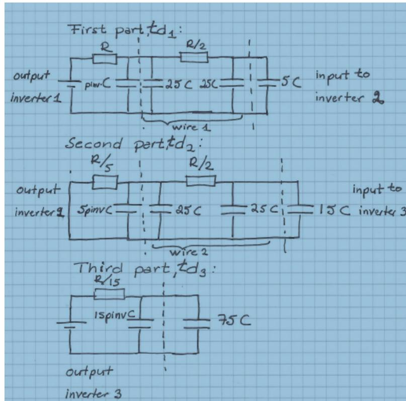
b) The corresponding delays, with  $p_{\text{inv}} = 1$ , are:
