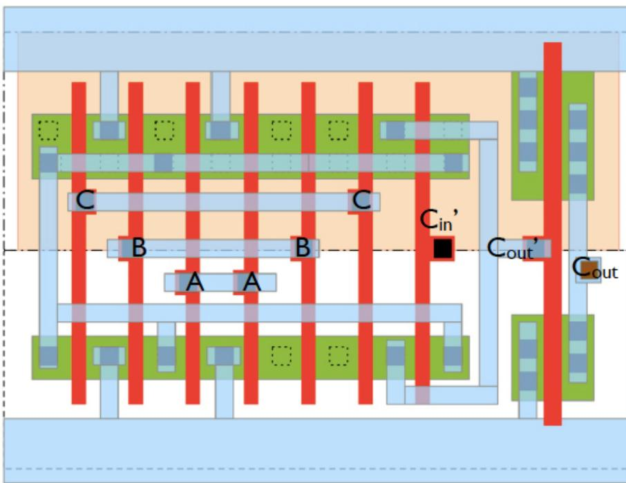
b) In the layout above there is only one p-diffusion drain area and one n-diffusion drain area connected to the output node so the parasitic delay for the circuit as it is laid out above is the same as that for an inverter.
