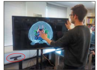
Figure 1.3: Microsoft’s Kinect interface can sense the user’s position and gestures, allowing a scientist to adjust the view of his data by “body language”, without a mouse or keyboard. (Data view courtesy of David Laidlaw; image courtesy of Emanuel Zgraggen.)
