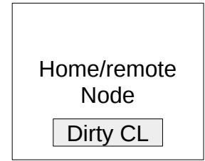
(e) The home node is different from the requesting node, the memory copy is dirty and the remote node is different from the home node
