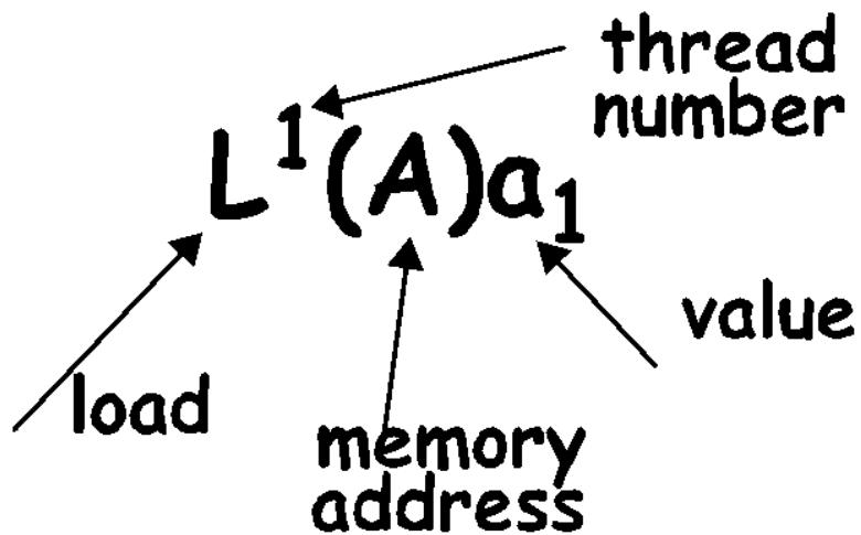
Load by thread T1 of address @A, loading the value  $a_1$
